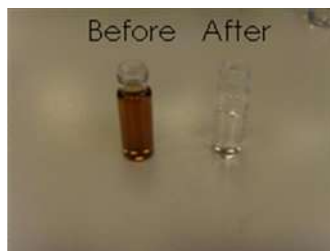
Comparison of the solution obtained before and after using AFFINIMIP® SPE Bisphenols
