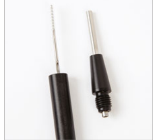
Figure 3: Cap removed, exposing probe tip brush for cleaning.
