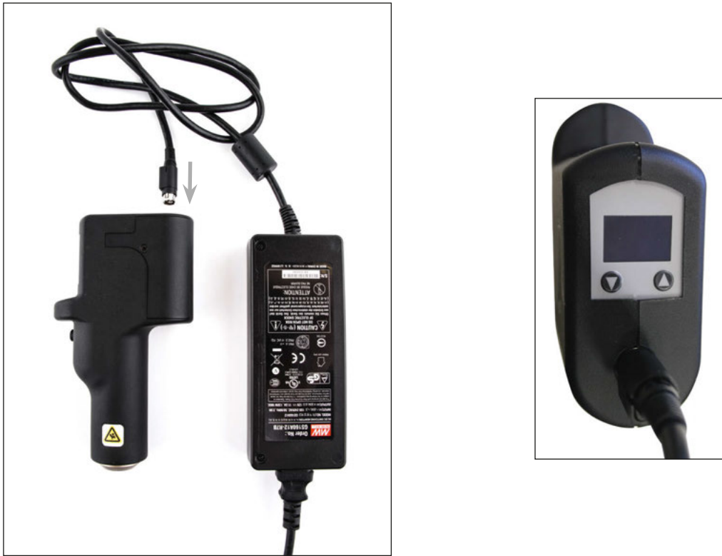
Figure 1. Power supply connector at the top of the HPS crimper
