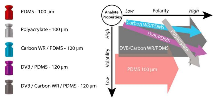
Color Code for easy optical identification of coating type and thickness
