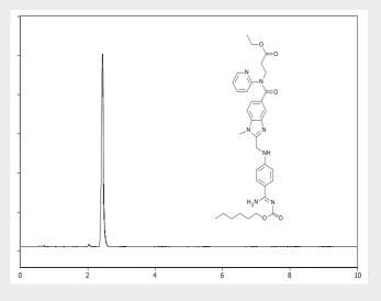
Column: 5µm SpeedCore C18 100x4.6mm Mobile Phase: 50:50 NH<sub>4</sub>OAc : ACN
