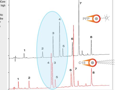
SpeedCore PFP columns will provide an alternative selectivity to that of traditional C18 reversed phased chemistries for the separation of basic, acidic and neutral species. PFP columns will retain by ion-exchange and shape selectivity mechanisms as well as both reversed and normal phase interactions. This makes them particularly useful for separation of closely related species such as isomers.
