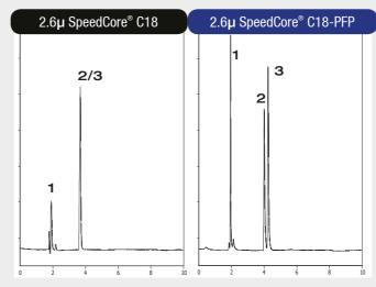
Column: 2.6µm SpeedCore C18 150x4.6mm 2.6µm SpeedCore C18-PFP 150x4.6mm Mobile Phase: 50:50 A:B A: 0.1% Formic acid B: MeOH Flow: 0.8ml/min Wavelength : 254nm 1. Benzene Sulphonic acid 2. Benzyl Alcohol
