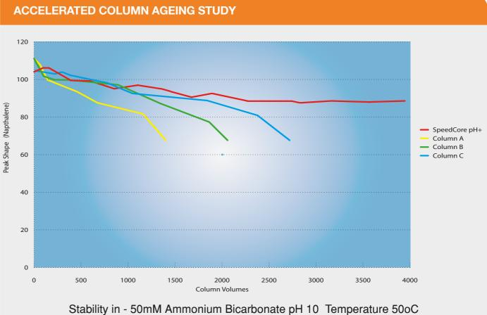
The first generation of core-shell particles suffered from short column lifetimes if run outside a moderate pH range of 2-8. As a result application of these columns was limited, as was the use of pH to achieve necessary selectivity and retention.
