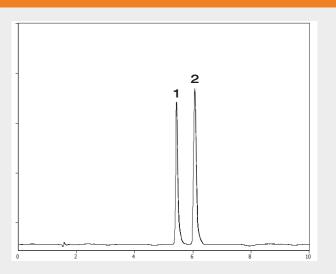
Column: 2.6µm SpeedCore C18-PFP 150x4.6mm Mobile Phase: 30:70 A:B A: 0.1% Formic acid B: MeOH Flow: 1.0ml/min Wavelength : 254nm
