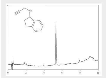
Column: 2.6µm SpeedCore C18 100x2.1mm Mobile Phase: A: 0.1% Formic acid B: ACN Gradient: 10-90%B in 10mins Flow: 0.4ml/min Wavelength : 254nm
