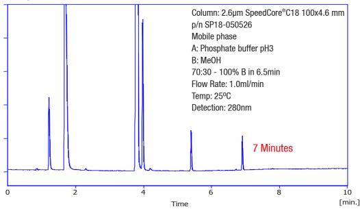
Method transfer using core-shell particles has moved the method from a 30 minute run time down to a 10 minute run time. A significant saving in time, money and solvent, with no lose of resolution. With a wide range of stationary phase choices now available on core-shell the analyst can potentially move all historical methods to the newer particles and save time and money.
