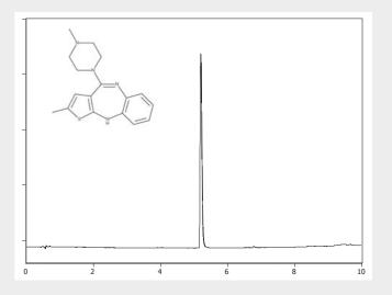
Column: 2.6µm SpeedCore C18 100x2.1mm Mobile Phase: A: 25mM NH<sub>4</sub>OAc B: ACN Gradient: 10-90%B in 10mins Flow: 0.4ml/min Wavelength : 254nm
