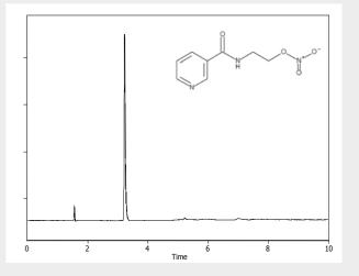
Column: 2.6µm SpeedCore RP18-Amide 150x4.6mm Mobile Phase: A: 10mM NH<sub>4</sub>OAc B: ACN Gradient: 20-100%B in 10mins Flow: 1.0ml/min Wavelength : 254nm
