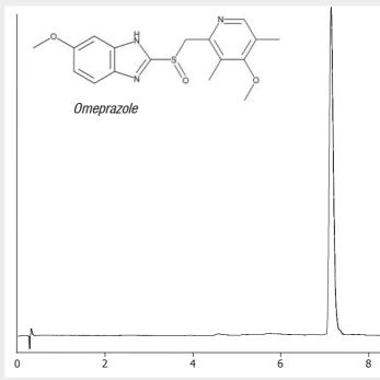
2.6µm SpeedCore pH+ 50x4.6mm A: 10mM Ammonium bicarbonate pH 10 B: MeOH Gradient: 60-80%B in 10mins Flow: 1.0ml/min Temp: 40°C Wavelength : 254nm 10 TRICYCLIC ANTIDEPRESSANTS 2.6µm SpeedCore pH+ 50x4.6mm Doxepin A: 10mM Ammonium bicarbonate pH 10 B: MeOH Gradient: 60-80%B in 10mins Flow: 1.0ml/min Imipramine Temp: 40°C Wavelength : 254nm Amitriptyline Trimipramine 5 pH 11
