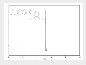
Column: 2.6µm SpeedCore RP18-Amide 150x4.6mm Mobile Phase: A: 10mM NH<sub>4</sub>OAc B: ACN Gradient: 20-100%B in 10mins Flow: 1.0ml/min Wavelength : 285nm
