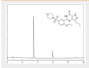
Column: 5µm SpeedCore C18 100x4.6mm Mobile Phase: A: 0.1% Formic acid B: ACN Gradient: 20-80%B in 10mins Flow: 1.2ml/min Wavelength : 230nm
