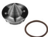
Skimmer cone, nickel, 0.9 mm orifice, 8003-0574
