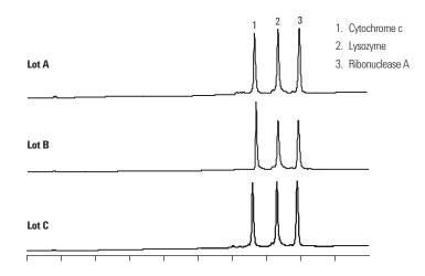
The combination of well-controlled resin production, column surface chemistry, and column packing virtually eliminates retention time variations from column-to-column and lot-to-lot.
