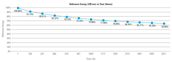
The Agilent-specific cathode coating process leads to less intensity drop over time, and extends lamp lifetime by more than 50%. All Agilent long-life deuterium lamps are guaranteed to have a lifetime greater than 2,000 hours.
