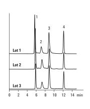
The four-protein mixture shows excellent retention time reproducibility over 300 injections and on three columns from different manufacturing lots.
