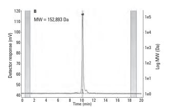
Comparison of traditional SEC analysis with UV detection and column calibration (A) and LS analysis at 90° (B) for anti-DYKDDDDK. Both MW results lie in the same range of approximately 153,000 Da.
