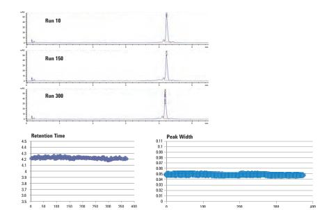
The ability to resolve oligonucleotides that differ by a single nucleotide is important for accurate characterization. The AdvanceBio Oligonucleotide column resolves N and N-1 for the Agilent Oligonucleotide Resolution Standard (14, 17, 20, and 21 mer).
