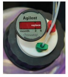
**Stay Safe caps** include a time strip that tells you when the venting valve needs to be replaced. We recommend changing the A-Line venting valve or the A-Line charcoal filter after six months of usage under the following conditions:
