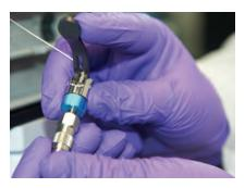
As easy as closing a lever: The proprietary Agilent design features a spring-loaded mechanism for zero dead volume and a sure, tight connection.
