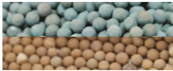
Moisture Adsorbent: Top: Full Capacity; Bottom: Depleted.
