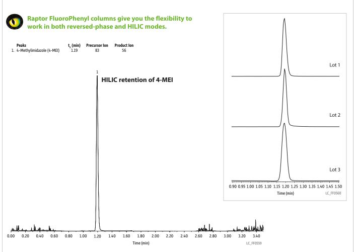
Column: Raptor FluoroPhenyl (cat.# 9319A52); Dimensions: 50 mm x 2.1 mm ID; Particle Size: 2.7 μm; Temp.: 35 °C; Sample: Diluent: Acetonitrile; Conc.: 100 ng/mL; Inj. Vol.: 5 μL; Mobile Phase: A: 0.1% Formic acid in water; B: 0.1% Formic acid in acetonitrile; Gradient (%B): 0.00 min (95% B), 2.00 (30% B), 2.01 (95% B); Flow: 0.6 mL/min; Detector: MS/MS; Ion Mode: ESI+; Mode: MRM; Instrument: UHPLC.
