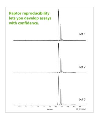
Column: Raptor FluoroPhenyl (cat.# 9319A1E); Dimensions: 100 mm x 3 mm ID, Particle Size: 2.7 µm; Temp.: 30 °C; Sample: Diluent: Water:methanol (50:50); Conc.: 25-50 ng/mL; Inj. Vol.: 5 µL; Mobile Phase: A: 0.1% Formic acid in water; B: Methanol; Gradient (%B): 0.00 min (75% B), 4.00 (85% B), 4.10 (100% B), 5.00 (100% B), 5.01 (75% B), 7.00 (75% B); Flow: 0.6 mL/min; Detector: MS/MS; Ion Mode: ESI+; Mode: MRM; Instrument: HPLC.
