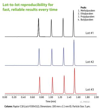
Column: Raptor Les (cat.# 9304512); Dimensions: 100 min x 2.1 min ib; Particle Size: 5 Jin; Temp.: 40 °C; Sample: Conc.: 100 µg/mL in water; Inj. Vol.: 1 µL; Mobile Phase: A: Water, B: Acetonitrile; Gradient (%B): 0.00 min (20% B), 2.00 min (80% B), 2.01 min (20% B), 3.50 min (20% B); Flow: 1.0 mL/min; Detector: PDA @ 254 nm; Instrument: UHPLC.
