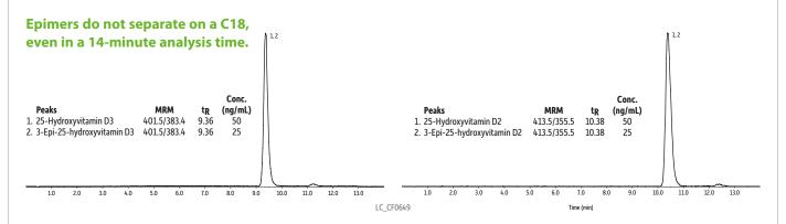
Column: Raptor ARC-18 (cat.# 9314A12); Dimensions: 100 mm x 2.1 mm ID, Particle Size: 2.7 µm; Temp.: 30 °C; Sample: Diluent: Water:methanol (50:50); Conc.: 25-50 ng/mL; Inj. Vol.: 5 µL; Mobile Phase: A: 0.1% Formic acid in water; B: Methanol; Gradient (%B): 0.00 min (75% B), 4.00 (80% B), 12.00 (80% B), 12.10 (75% B); 14.00 (75% B); 14.00 (75% B); 15 mL/min; Detector: MS/MS; Ion Mode: ESI+; Mode: MRM; Instrument: HPLC.
