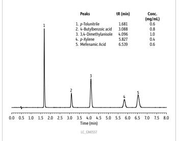
Column: Raptor C18 (cat.# 9304A1E); Dimensions: 100 mm x 3 mm ID; Particle Size: 2.7 μm; Pore Size: 90 Å; Temp.: 30 °C; Sample: Diluent: Acetonitrile:water:phosphoric acid (65:34:1); Inj. Vol.: 1 μL; Mobile Phase: A: 0.05% Formic acid in water, B: 0.05% Formic acid in acetonitrile; Gradient (%B): 0.00 min (45% B), 8.00 min (45% B); Flow: 0.8 mL/min; Detector: UV/Vis @ 220 nm; Cell Temp.: 40 °C: Instrument: HPLC.
