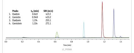
Column Force C18 (cat.# 9634252), Dimensions:50 mm x 2.1 mm ID, Particle Size: 1.8 µm, Temp.: 50 °C, Sample Custom mix, Diluent: Water, Inj. Vol.: 2 µt; Mobile Phase A: Water + 0.1% formic acid, B: Acetonitrile + 0.1% formic acid; Gradient (%B): 0.00 min (15%), 1.50 min (95%), 1.51 min (15%), 3.00 min (15%); Flow: 0.6 mL/min; Max Pressure: 500 bar; Detector: MS; Interface: E51+; Instrument: UHPLC.
