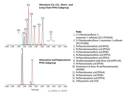
Column: Raptor Polar X (cat.# 9311A52); Dimensions: 50 mm x 2.1 mm ID, Particle Size: 2.7 μm; Temp.: 40 °C; Sample: Diluent: 50:50 Water:-methanol; Conc.: 400 ng/L; Inj. Vol.: 10 μL; Mobile Phase: A: Water, 10 mM ammonium formate, 0.05% formic acid; B: 60:40 Acetonitrile:methanol, 0.05% formic acid; Gradient (%B): 0.00 min (85% B),8.00 min (85% B); Flow: 0.5 mL/min; Detector: MS/MS; Ion Mode: ESI-; Mode: MRM; Instrument: UHPLC.
