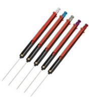
Due to the relatively large diameter of PAL Smart SPME Arrows, you must modify the GC inlet using an instrument-specific conversion kit from Restek prior to use. Converted inlets are compatible with all standard injection techniques (SPME Arrow, liquid syringe, headspace, etc.); no need to switch inlets after installation.
