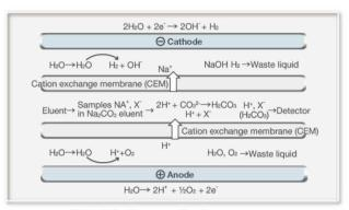
Principle diagram of anion suppressor
