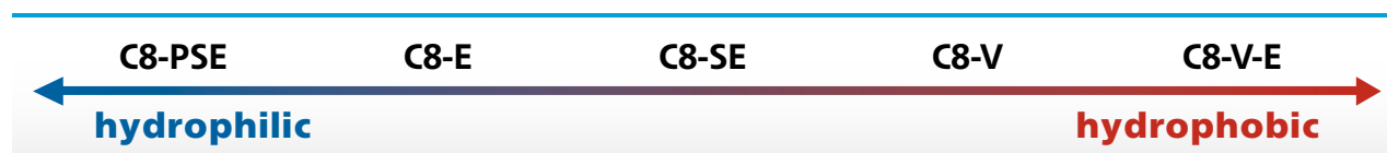
Figure 1: Hydrophobicity of VDSpher® OptiBio (300 Å) C8 modifications
