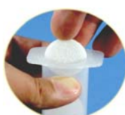
Frit (thick) insertion
